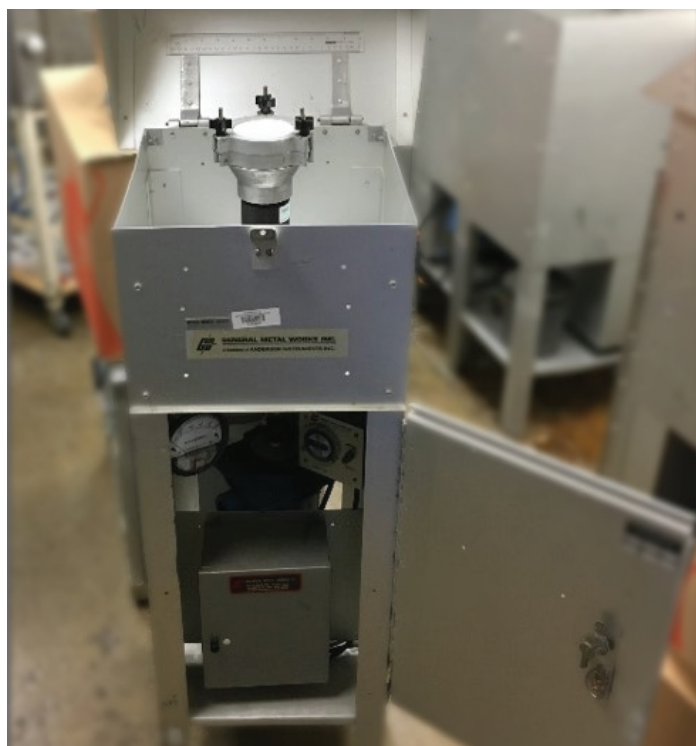
PS-1 high-volume air sampler with media installed
