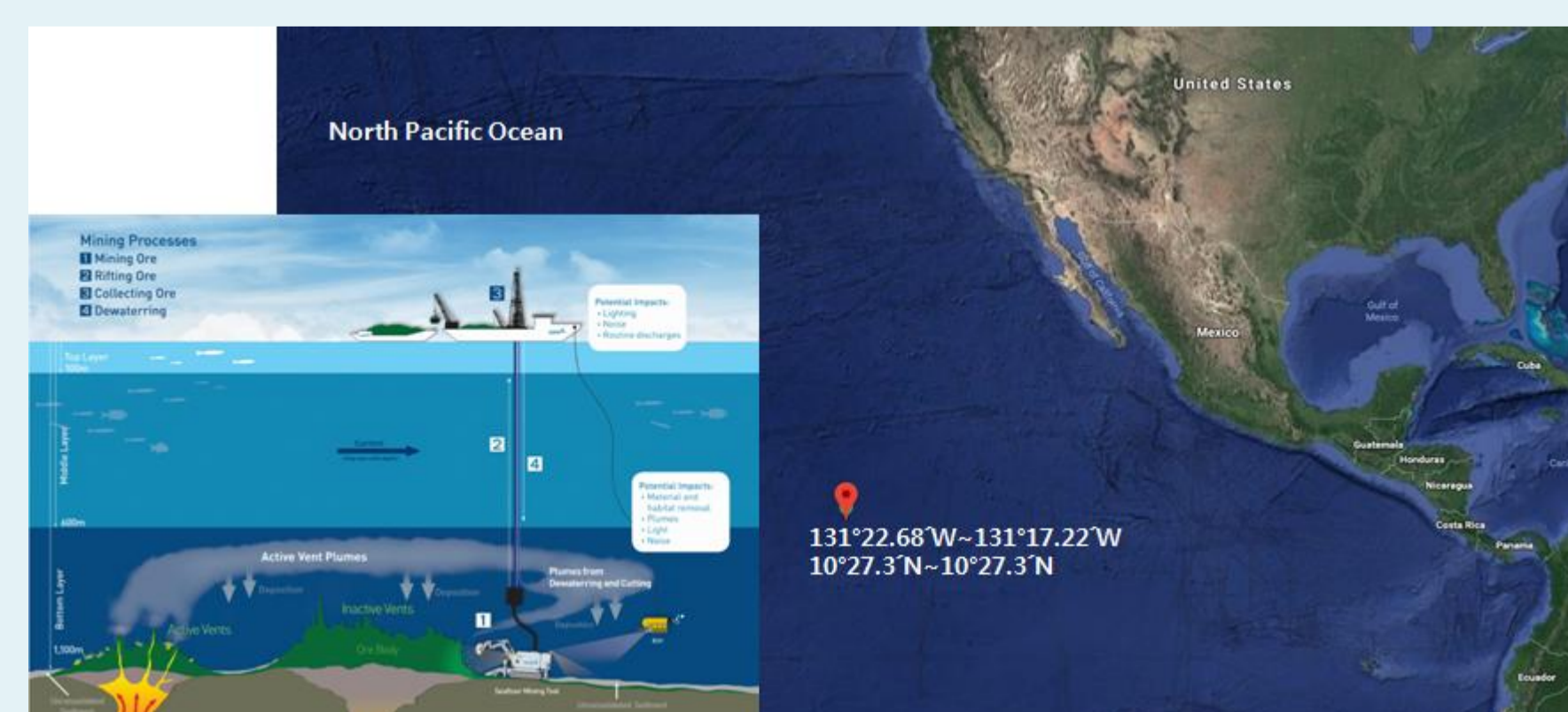
Figure 1. Schematic diagram of deep-sea mining process and collecting area map of polymetallic nodules
