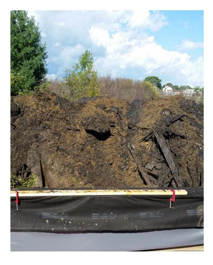
The material initially dredged from the river contained a significant amount of wood chips and smaller woody particles and required a considerably larger quantity (>20%) of amendment than anticipated to solidify the sediment to "pass" the paint filter test.
