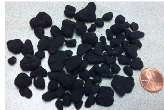
Figure 1. Configuration of PAC-coated particle.
