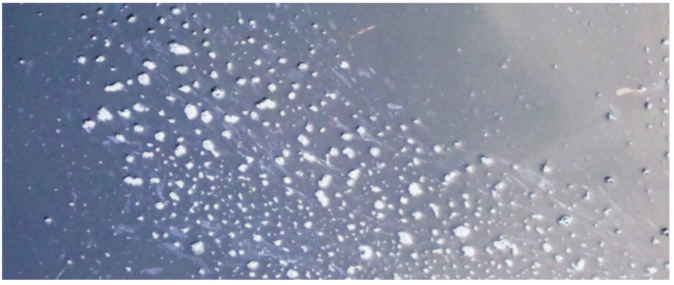
FIGURE 1. PCB Oil Sheen Observed On Water Surface During Phase 1 Dredging.
