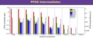
PFOS decomposition yields formation of PFCAs found in the effluent (LC-MS/MS) followed by chain shortening, including C2-C6 PFCAs. DRE > 99.999% at 650 °C
