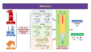
Supercritical water oxidation (SCWO) leverages high temperature, high pressure, and high oxidative radical concentrations to destroy PFAS and organic contaminants
