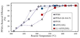
Landfill Leachate + AFFF matrix is the most recalcitrant of tested compounds. Temperature of >610 °C is required -- higher that neat PFOS or AFFF.
