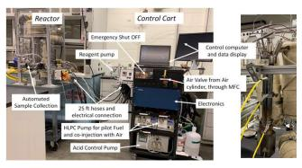
Autogenic operation is established by custom control hardware and software. Control of pilot fuel (ethanol) and air flow rate determine temperature and the residence time.
