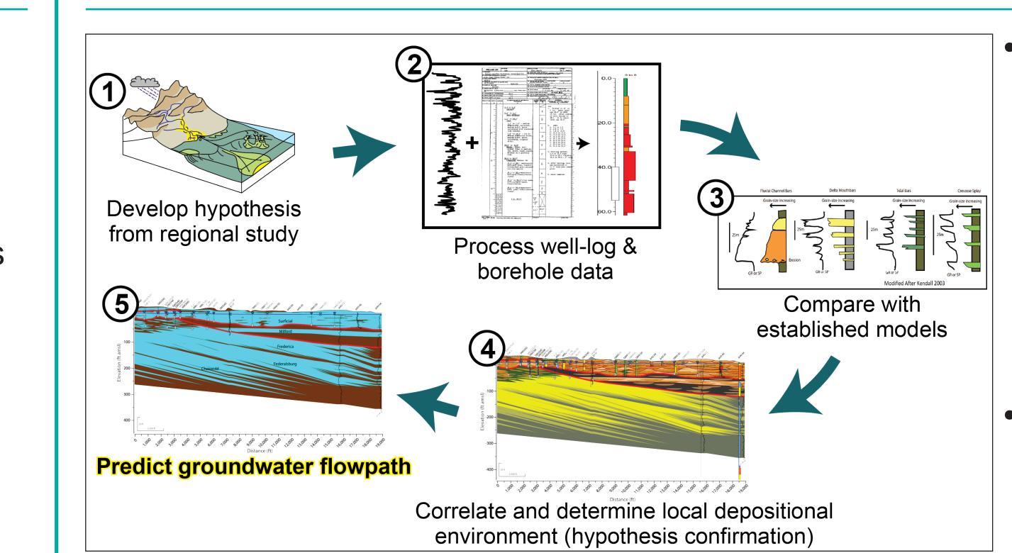
Figure 1. Predictive Integrated Stratigraphic Modeling (PRISM®)
