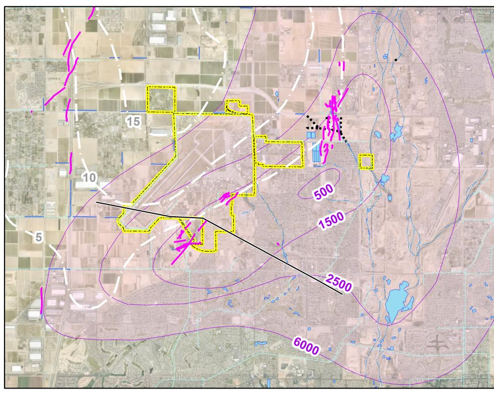
Regionally subsidence due to aquifer compaction has been greater than 15 feet. Subsidence due to over pumping is common in the American SW; however, earth fissures are an uncommon occurrence.
