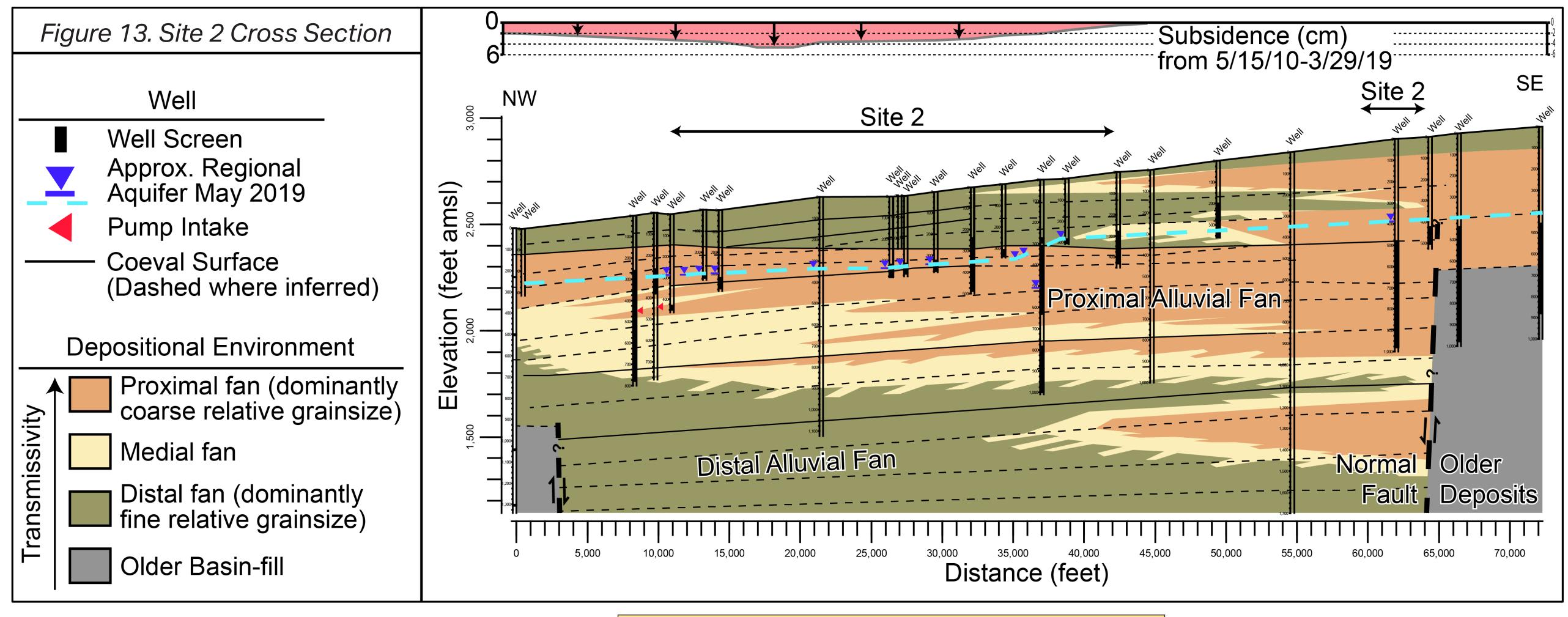
Surface waters within ditches delivered relatively little impacted water to the subsurface until reaching a source-distant unlined retention pond. Ephemeral surface waters drove the constituents vertically through the vadose zone to the groundwater table where a stratigraphic analysis showed that migration was focused within a single alluvial fan lobe. This review offered the client a targeted area of remediation for surficial soils and groundwater.
