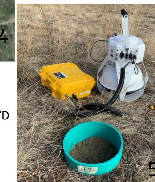
Figure 5. Dynamic closed chamber with infrared gas analyzer.
