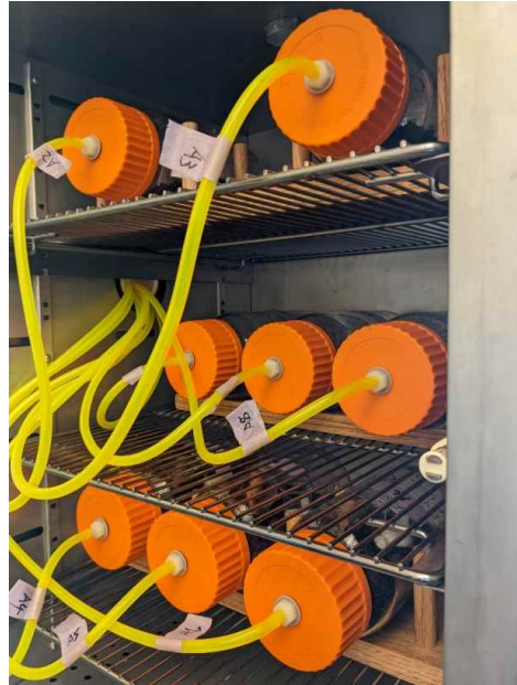
Respirometer can monitor eight soil samples simultaneously
