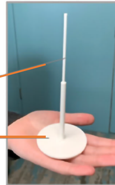
3-D printed rotary shaft and spinning disk
