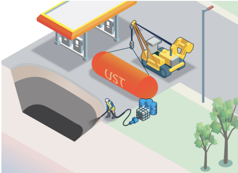
Spray applications when USTs or piping are removed
