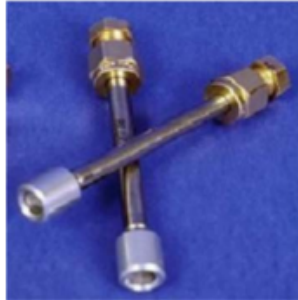
Passive diffusion samplers, shown here, replaced Summa canisters. These devices are designed to collect a sample over a period of 14 to 26 days. Research has shown that a long-duration sample is more effective at determining if vapor intrusion is occurring in a home than a 24-hour sample.
