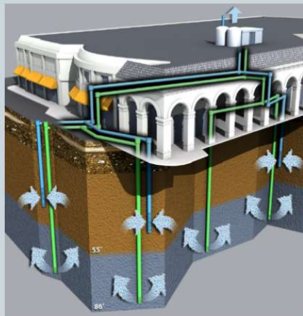
Air Sparging/SVE System
