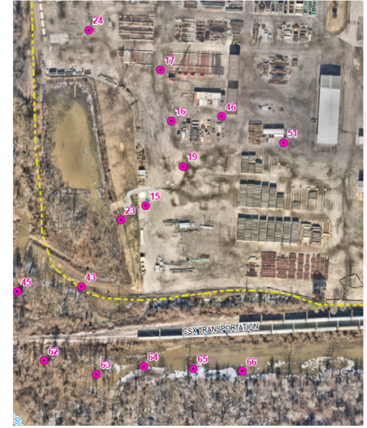
Exhibit 6 CPT boring locations.
