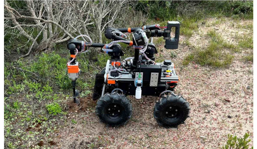
Image 1: Photo of Robot Used for Excavation Monitoring
