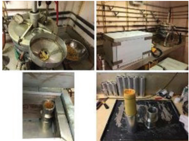
Figure 1: Explosive melt-cast preparation at Battelle
